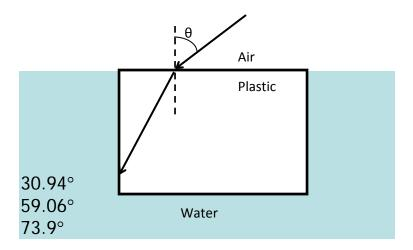
A light beam is incident at an angle  $\theta$  on the top surface of a block of plastic. Find the maximum value of  $\theta$  for which the refracted light is totally reflected from the left face of the plastic block, if the block is immersed in water. ( $n_{plastic}=1.49$ ,  $n_{water}=1.33$ ).
