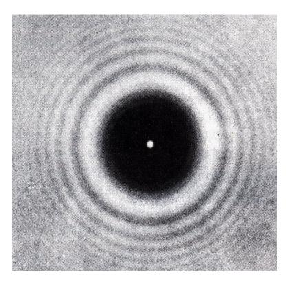
The central bright spot is a result of light "bending" around the edges of the penny and interfering constructively in the exact center of the shadow.
