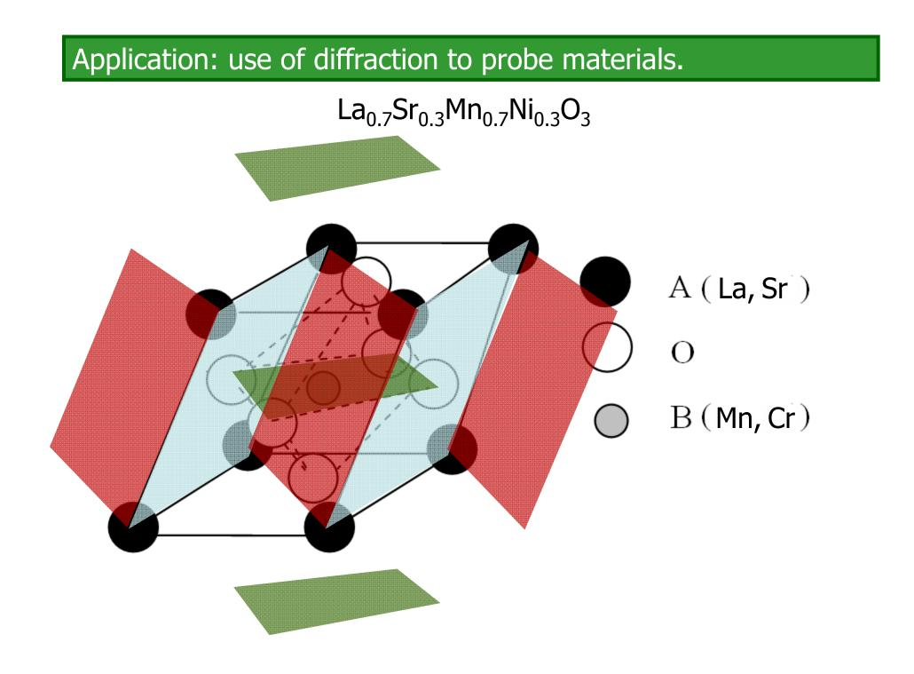
Application: use of diffraction to probe materials.
