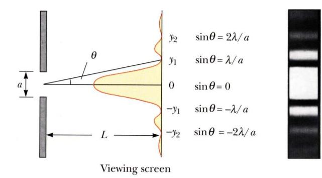
Most of the intensity is in the central maximum. It is twice the width of the other (secondary) maxima. Starting equations for single-slit intensity:
