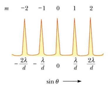
The intensity maxima are brighter and sharper than for the two slit case. See <u>here</u> and <u>here</u>.
