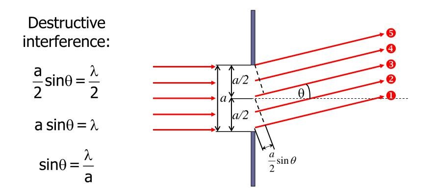
If you divide the slit into 4 equal parts, destructive interference occurs when  $\sin\theta = \frac{2\lambda}{a}$ .
