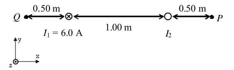
Two long parallel conductors are separated by 1.0 m. The wire on the left carries a current  $I_1 = 6.0$  A into the page. (c) If a third long wire is placed at P and carries a current  $I_3 = 2.0$  A in the –y direction, what is the magnitude and direction of the net magnetic field at point Q?
