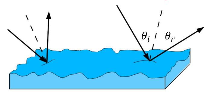
Angle of incidence equals angle of reflection.
