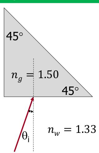
Example: a  $45^{\circ} - 45^{\circ} - 90^{\circ}$  glass (n = 1.50) prism is surrounded by water (n = 1.33). Light is incident at a  $23^{\circ}$  angle, as shown in the diagram. What angle does the light make when it exits the prism?
