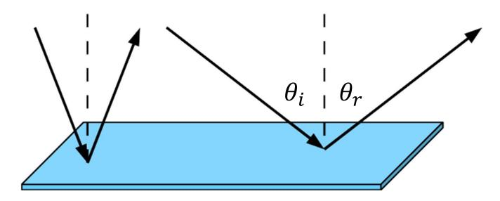
Angle of incidence equals angle of reflection.
