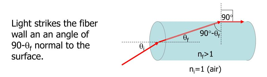
At the critical angle, instead of exiting the fiber, the refracted light travels along the fiber-air boundary. In this case,  $90^{\circ}-\theta_{f}$  is the critical angle.
