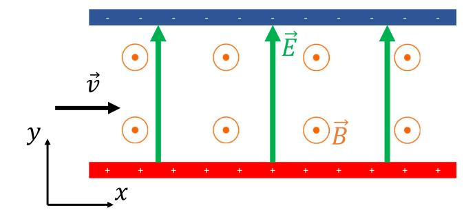
Example: Alpha particles ( $m_{\alpha} = 4m_p$ ,  $q_{\alpha} = 2e$ ) are accelerated through a potential difference,  $V_0$ , and then pass through a magnetic field perpendicular to their velocity. What magnetic field (magnitude and direction) should be used to produce a radius of curvature, R, in the direction shown?
