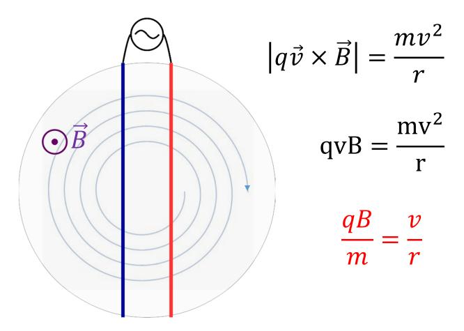
Particles spiral out as they accelerate, increasing speed and radius proportionally so that the period and frequency
