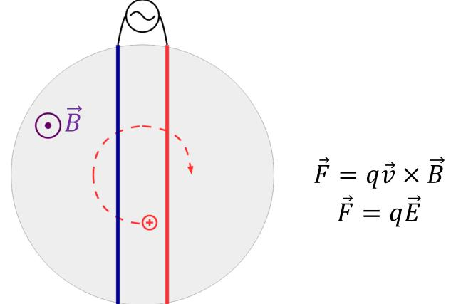
Particles spiral out as they accelerate, increasing speed and radius proportionally.
