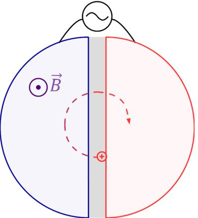
Instead of plates, use "D's", hollow *D*-shaped conductors with a top, a bottom and an outside edge.
