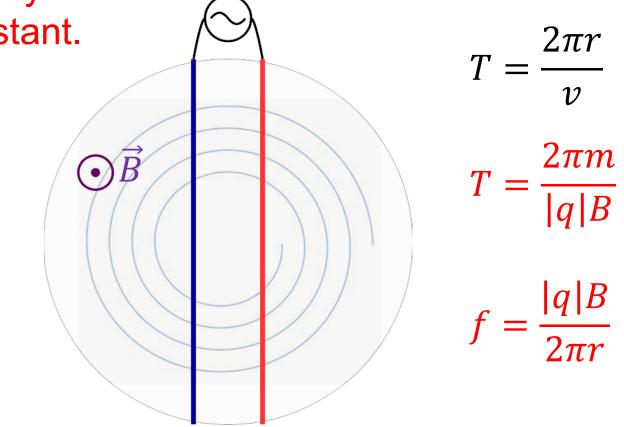
Instead of plates, use "D's", hollow D-shaped conductors with a top, a bottom and an outside edge.
