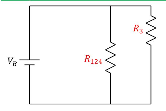
$R_{1} = 60\Omega$  $R_{2} = 40\Omega$  $R_{3} = 75\Omega$  $R_{4} = 26\Omega$  $V_{B} = 24V$  $R_{12} = 24\Omega$  $R_{12} = 50\Omega$
