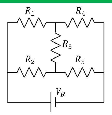
$R_1 = 30\Omega$  $V_1 = 24V$  $V_2 = 36V$  $R_2 = 90\Omega$  $R_3 = 40\Omega$  $V_3 = 12V$  $R_4 = 52\Omega$  $V_4 = 26V$  $R_5 = 20\Omega$  $V_{5} = 14 V$  $R_T = 42\Omega$  $V_{B} = 50V$  $I_1 = 0.8A$  $I_2 = 0.4$ A  $I_3 = 0.3A$  $I_4 = 0.5A$  $I_5 = 0.7 A$  $I_{T} = 1.2A$
