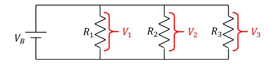
$$V_T = V_1 = V_2 = V_3$$
