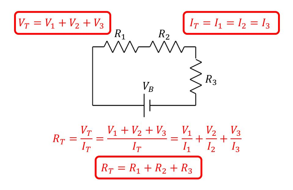
$$V_T = V_1 + V_2 + V_3$$
