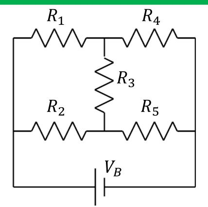
$V_B = 50V$  $R_1 = 30\Omega$  $R_2 = 90\Omega$  $R_3 = 40\Omega$  $R_4 = 52\Omega$  $R_5 = 20\Omega$
