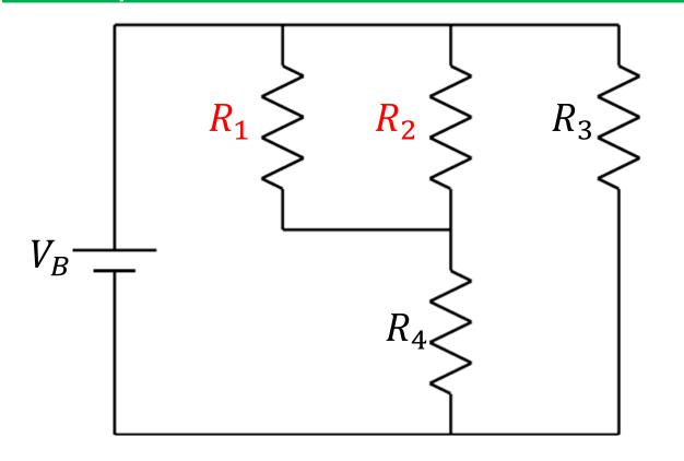
$R_1 = 60\Omega$  $R_2 = 40\Omega$  $R_3 = 75\Omega$  $R_4 = 26\Omega$  $V_B = 24V$
