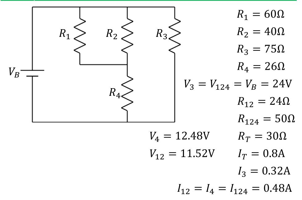
Example: Consider the given circuit.(a) Determine the total (equivalent) resistance.(b) Determine the total current.(b) Determine the potential difference across each resistor.
