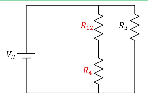
$R_{1} = 60\Omega$  $R_{2} = 40\Omega$  $R_{3} = 75\Omega$  $R_{4} = 26\Omega$  $V_{B} = 24V$  $R_{12} = 24\Omega$
