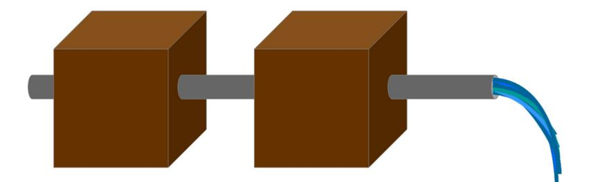
A set of pipes in series is more resistant to flow than any of the individual pipes in the series.
