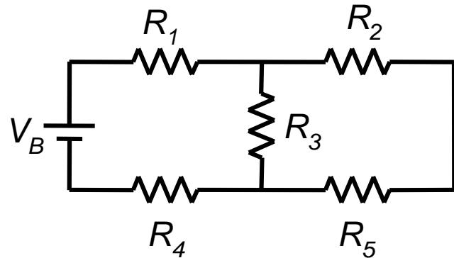
Note that  $V_{325} = V_3 = V_{25}$ .
