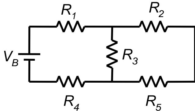
Note that  $V_3 = V_2 + V_5$
