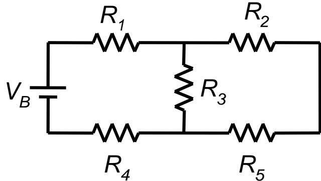
$$R_T = R_1 + R_{325} + R_4$$
