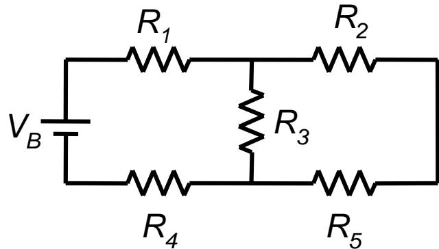
$$R_{25} = R_2 + R_5$$
