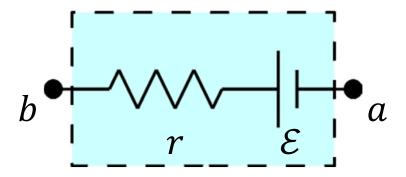
$\mathcal{E}$  is the ideal V of the battery. r is the internal resistance of the battery.  $V_{ab}$  is the real V of the battery.
