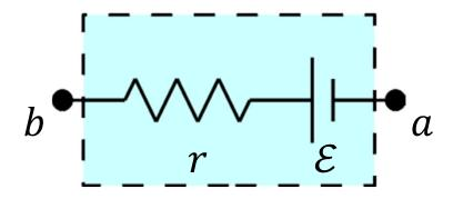
Can only measure terminal voltage,  $V_{ab}$ .
