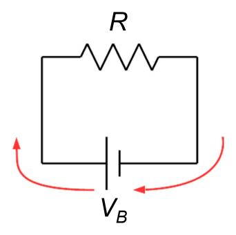
Charges leaving the battery have more energy than charges entering battery. Consider  $V = \frac{U}{q}$   $V_{\text{Leaving}} = V_{\text{Entering}} + V_{B}$
