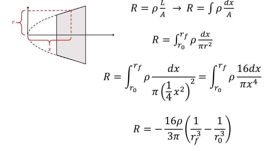
Example: The radius of a conductor is given by  $r = \frac{1}{4}x^2$ between x = 2mm and x = 4mm. Determine the resistance of the conductor for a current flowing in the *x*direction.
