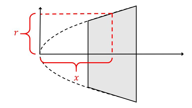
Example: The radius of a conductor is given by  $r = \frac{1}{4}x^2$ between x = 2mm and x = 4mm. Determine the resistance of the conductor for a current flowing in the *x*direction.
