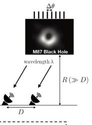
The radio wave can penetrate interstellar dust clouds and hence reach us. EHT adopts two frequency bands, 230GHz and 345GHz.
