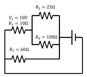
(10) a. Determine  $R_T$ , the total equivalent resistance of the circuit.
