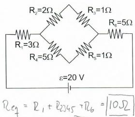
$$\overline{I}_{23} = \frac{V_{23}}{R_{23}} = \frac{4V}{3\Omega} = \frac{4}{3}A \qquad \widehat{P}_{3} = \overline{I}_{3}^{2}R_{3} = \left(\frac{4}{3}A\right)^{2}I\Omega = \boxed{\frac{16}{9}W}$$
