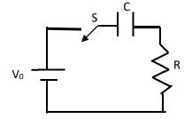
(10) (a) At time t = 0 the switch S is closed and the capacitor starts to charge. Determine the final charge on the capacitor after a very long time.
