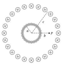
(15) b. Beginning with Ampere's Law, determine the magnitude of the magnetic field at point *P*.
