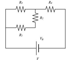
(15) a. Calculate the equivalent resistance of the entire circuit.
