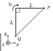
(15) c. Determine the magnetic force on the portion PQ. Give an answer in a vector notation.
