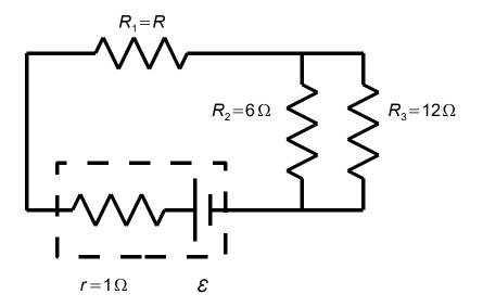
(10) (a) If the current through  $R_3$  is 1A, find the current  $I_2$  through resistor  $R_2$ .
