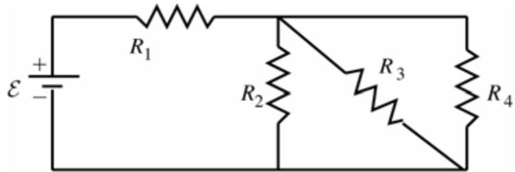
(a) (10 points) Find the equivalent resistance of the resistors connected across the power supply.
