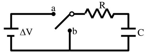
(a) (5 points) At  $t=0$ , the switch is thrown to position a. What is the current through the resistor immediately after the switch is thrown to position a?
