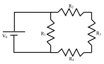
(20) b) The power supply provides a potential difference  $V_0 = 18 \text{ V}$ . Determine the power dissipated by resistor  $R_4$ .
