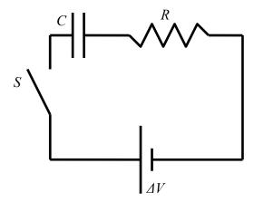
(30) b) After the switch has been closed for time *T* the voltage across the capacitor is found to be 1/5 of its final value. Find *R*? You should express your answer in terms of system parameters (do not attempt a numerical solution).
