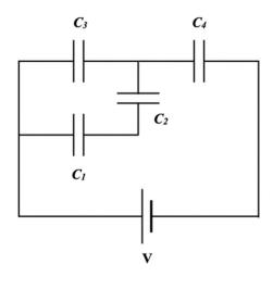
(10) a. Calculate  $C_T$  the equivalent capacitance of the entire circuit.
