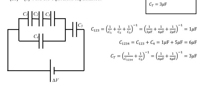
(20) (b) If the charge on  $C_3$  is 12  $\mu$ C find  $\Delta V$ .
