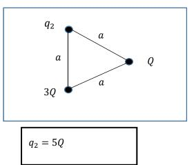
(10) (b) Determine the electric potential at the location of  $q_2$ . (Assume  $q_2$  is not present.)
