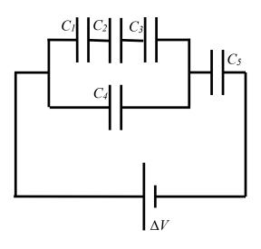
(20) (b) If the charge on  $C_3$  is 12  $\mu$ C find  $\Delta V$ .
