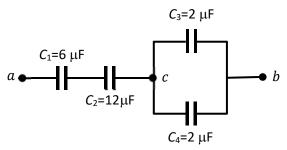
(15) (a) Calculate the total (equivalent) capacitance of this configuration of capacitors.
