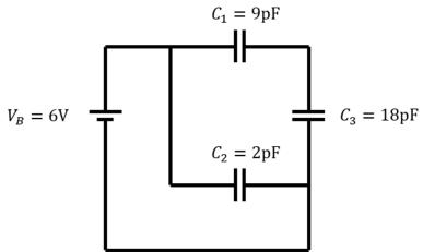
(15) (a) Determine  $C_T$ , the total equivalent capacitance.
