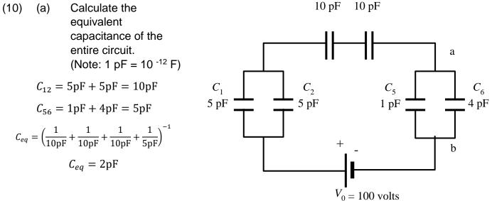
(10) (b) Find the charge  $Q_3$  on capacitor  $C_3$ .  $Q_3 = Q_{eq} = C_{eq}V_0 = (2\text{pF})(100\text{V}) = 200\text{pC}$
