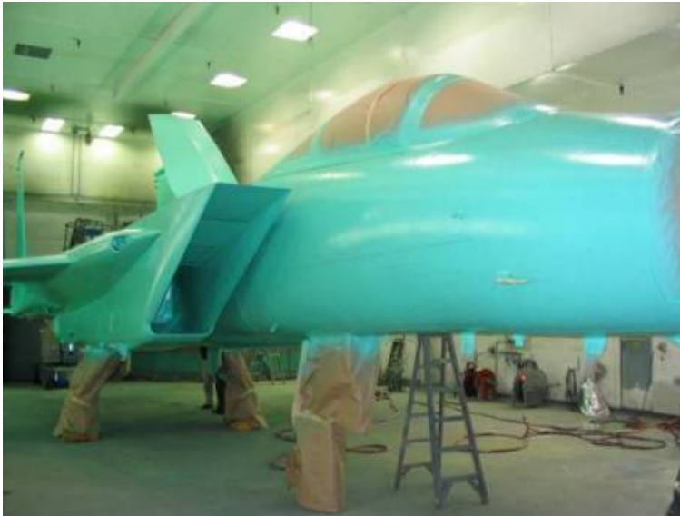
F-15 coated with Deft 02GN084 non-chromate primer that uses a Pr-based inhibitor
