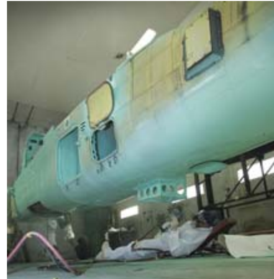
Technician coating an Apache fuselage with Deft non-chrome primer
